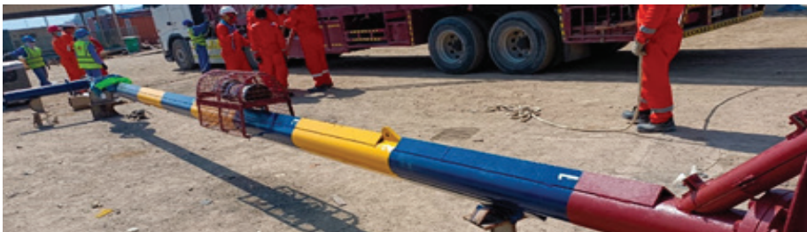
FABRICATION OF USBL PIPE FOR UNDERWATER POSITIONING SYSTEM.
