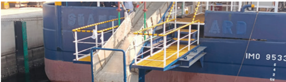
FABRICATE & INSTALLED AFT SHEAVE SLIPWAY WITH WALKWAY PLATFORM FOR NODE HANDLING.
